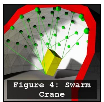
designed around cranes. By removing this design criteria, buildings will naturally take the shape of domes, which are more rigid and better suited for maintaining internal environmental conditions. This, in turn, will allow vast internal volumes free from supports, which will synergize with on-site monolithic manufacturing of large products such as aircraft.
